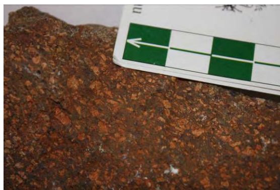
Figure 10.1. Photo of hand sample of McGregor Volcanics (2008371045), showing undeformed volcanic texture. Bars on scale are 1 cm.
