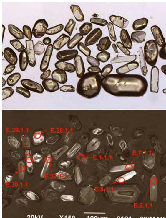
Figure 63.2. Representative transmitted light and cathodoluminescence images of zircons from the Hodgkinson Granodiorite (2007379005), with locations of some SHRIMP analyses.
