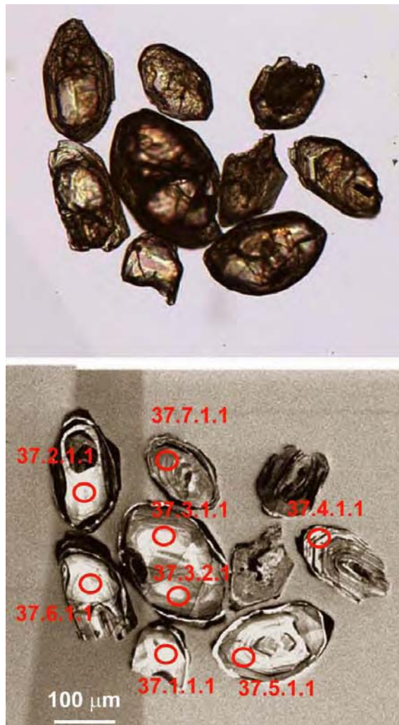
Figure 30.2. Representative transmitted light and cathodoluminescence images of zircons from the Carpa Granite (2008371037), with locations of some SHRIMP analyses.
