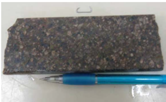
Figure 67.1. Porphyritic unnamed granite from the 482 m to 488 m depth interval of drill hole BRD 012 (sample 2009371038), with a pen for scale.
