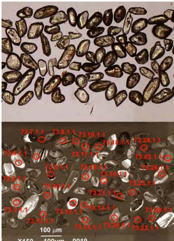
Figure 6.2. Representative transmitted light and cathodoluminescence images of zircons from the Broadview Schist (2008371073), with locations of some SHRIMP analyses.
