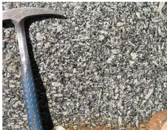
Figure 60.1. Grey, coarse-grained granite of the Yerila Granite, from southwest of Mount Babbage, Mount Babbage Inlier (sample 2007379013).
