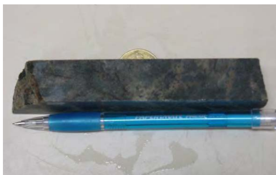
Figure 64.1. Unnamed calc-silicate from the 414 m to 418.9 m depth interval of drill hole SPH 1 (sample 2009378027), with a pen for scale.
