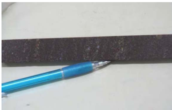
Figure 66.1. Red sandstone from the 469.3 m to 474.6 m depth interval of drill hole Bumbarlow 1 (sample 2009378006), with a pen for scale.
