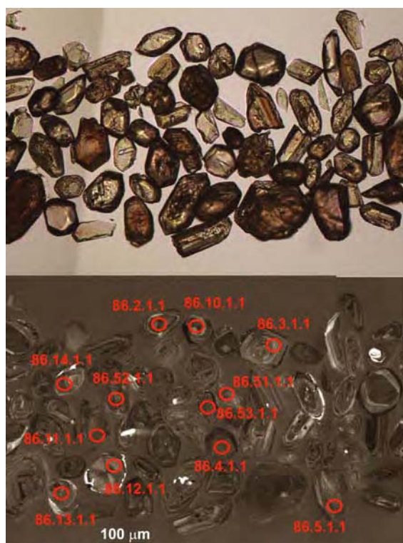
Figure 14.2. Representative transmitted light and cathodoluminescence images of zircons from the Cooyerdoo Granite (2008371086), with locations of some SHRIMP analyses.
