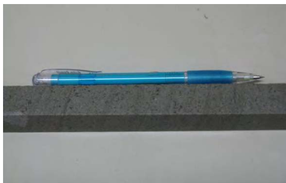
Figure 65.1. White sandstone from the 686 m and 691 m depth interval of drill hole Bumbarlow 1 (sample 2009378001), with pen for scale.
