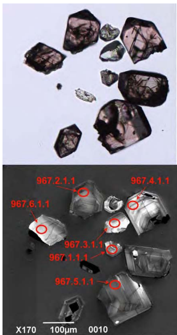
Figure 68.2. Representative transmitted light and cathodoluminescence images of zircons from the unnamed metasediment, ETMA5 1 drillhole (2009378018), with locations of some SHRIMP analyses.
