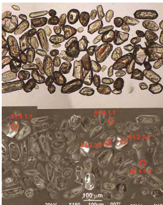
Figure 19.2. Representative transmitted light and cathodoluminescence images of zircons from leucogranite north of Lake Gilles (2008371081), with locations of some SHRIMP analyses.
