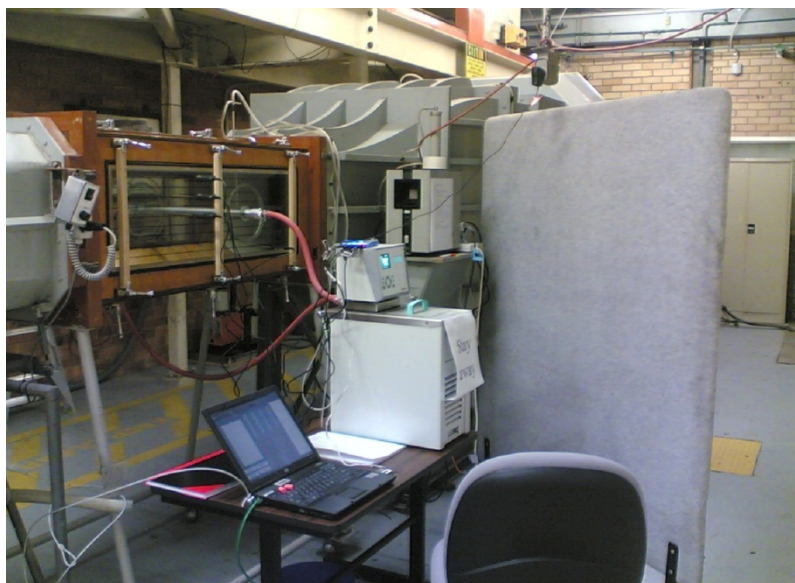
Figure 6 The low speed wind tunnel test facility; the test section
