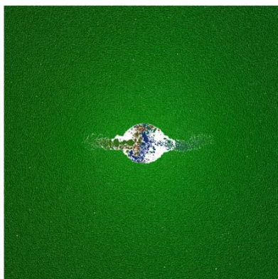
Figure 4 Development of compaction breakout. Long and narrow slot-shaped breakouts are observed, perpendicular to the major compressive stress \sigma_H
