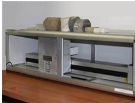
Figure 2. Field optical scanning instrument for rock thermal property measurements on full size cores.
