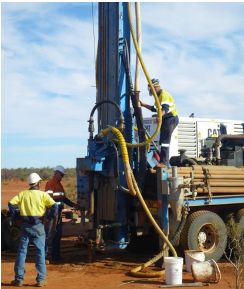
Figure 3. Reverse Circulation (RC) drilling into buried palaeovalleys that had been defined by gravity profiling.
