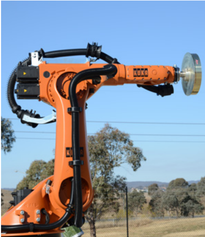
Figure 4: Robots are used to calibrate GNSS antennas and improve how accurately we can measure the dynamic Earth.
