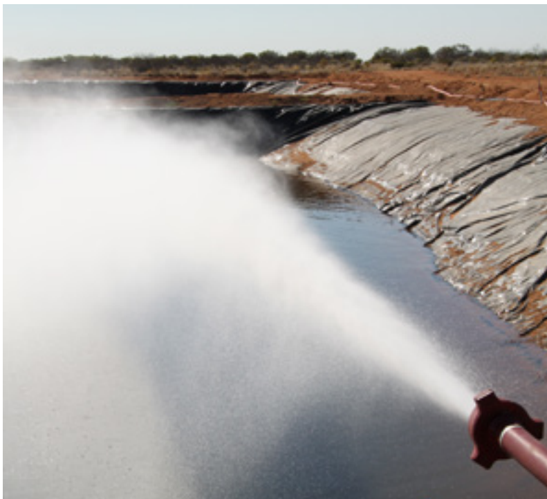
Figure 2: Water flowing from the Paralana-2 open well flow test. Courtesy Petratherm Ltd.
