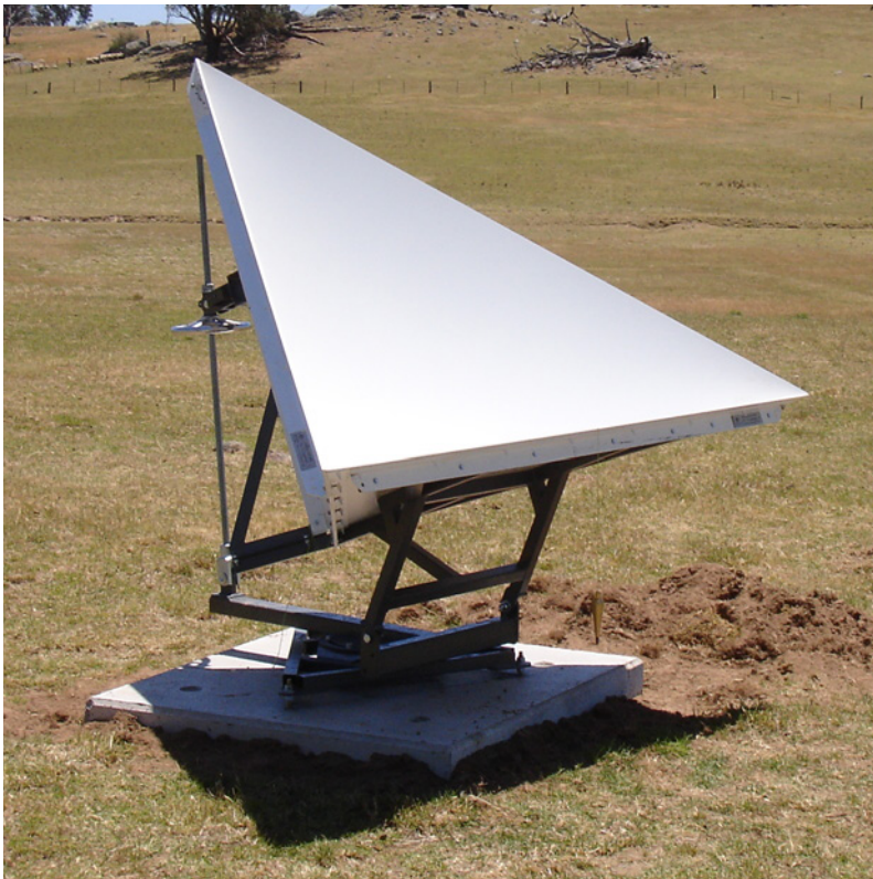
Figure 1. Corner reflector deployed at a test site north of Canberra.
