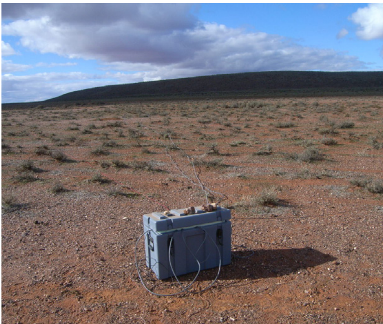
Figure 2. An AusLAMP MT station set-up for continuous recording of electric and magnetic signals in the field.
