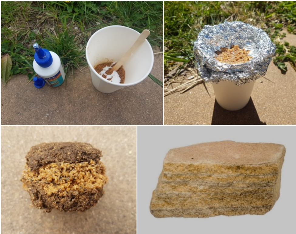
Figure 3: Mixing glue and sand in a cup, sand layer setting in a foil-lined cup, new glued sandstone rock, real layered sandstone.
