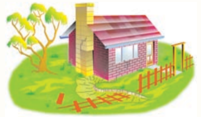
Tilted fences and cracks in buildings are indicators of potential hazards.
