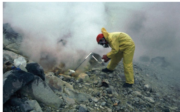
Figure 9: A volcanologist collects volcanic gasses. Notice the use of a respirator mask and hazardous materials suit due to the poisonous vapours, and a helmet in case of flying rocks! Source: USGS http://volcanoes.usgs.gov/Images/Jpg/Monitoring/Gas/GasMageik_large.jpg
