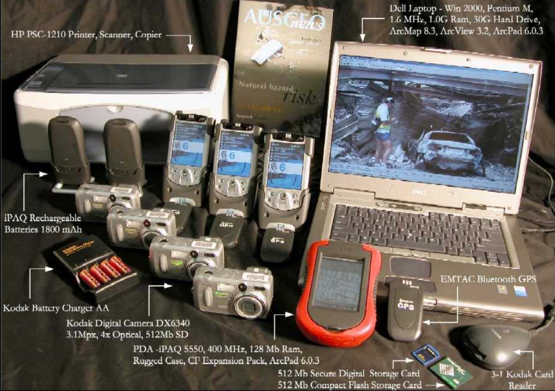
Equipment used by GA fieldwork teams to collect pre and post-hazard information. Image courtesy Geoscience Australia.
