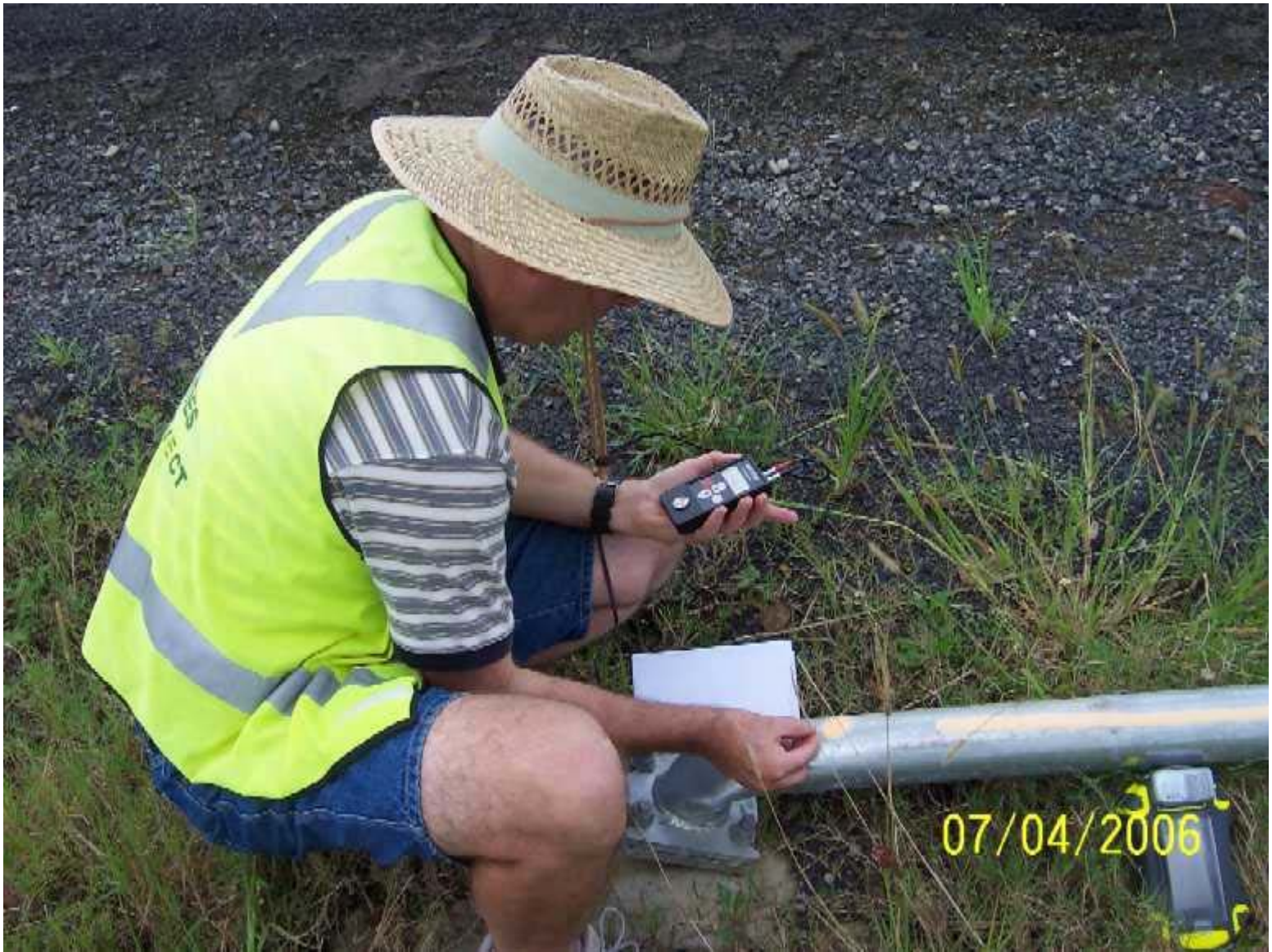
Calculating the wind speed of Cyclone Larry by measuring the damage to steel posts. Image courtesy Geoscience Australia.
