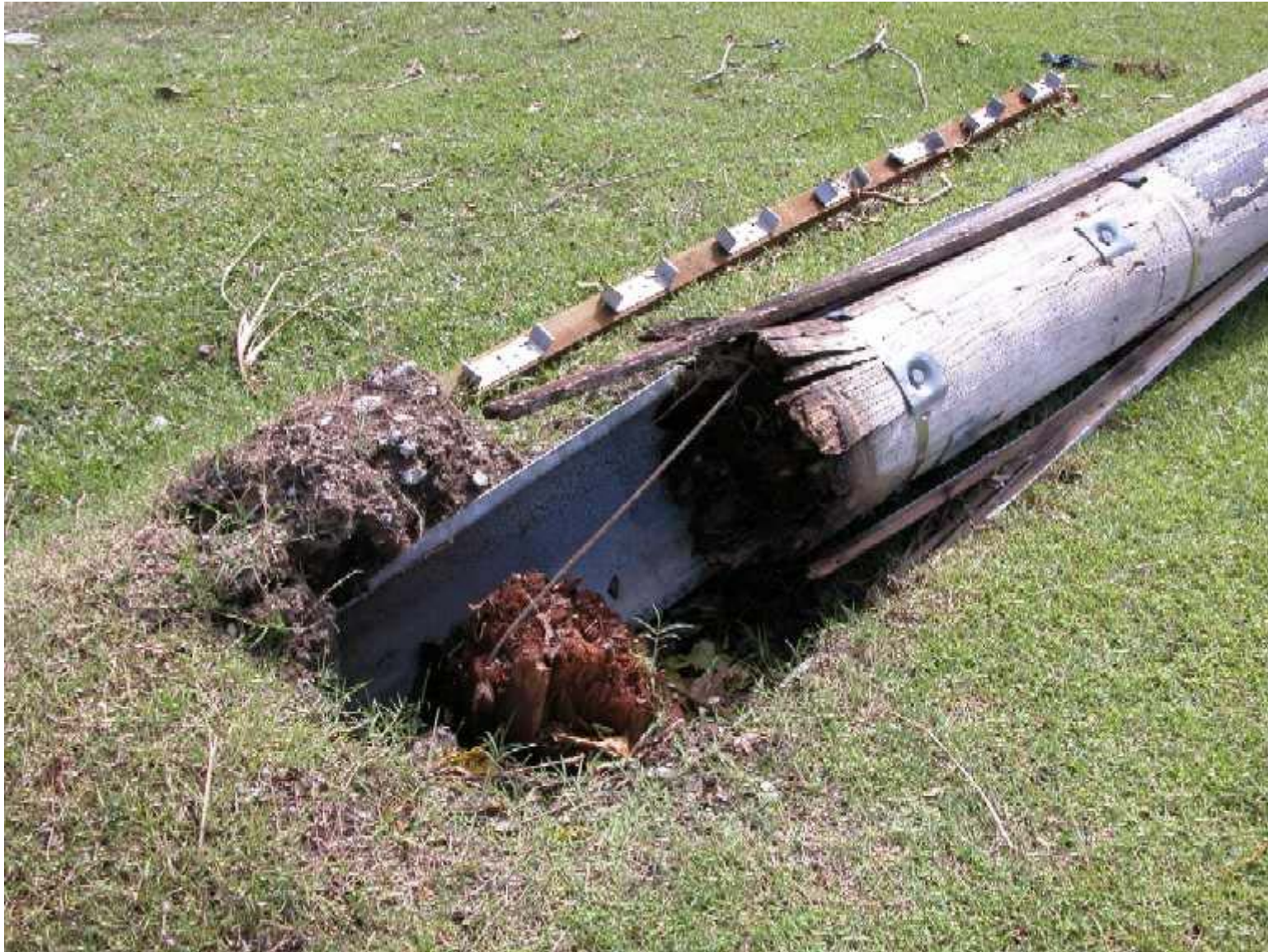
Damage to a power pole in Innisfail following Cyclone Larry. Image courtesy Geoscience Australia.
