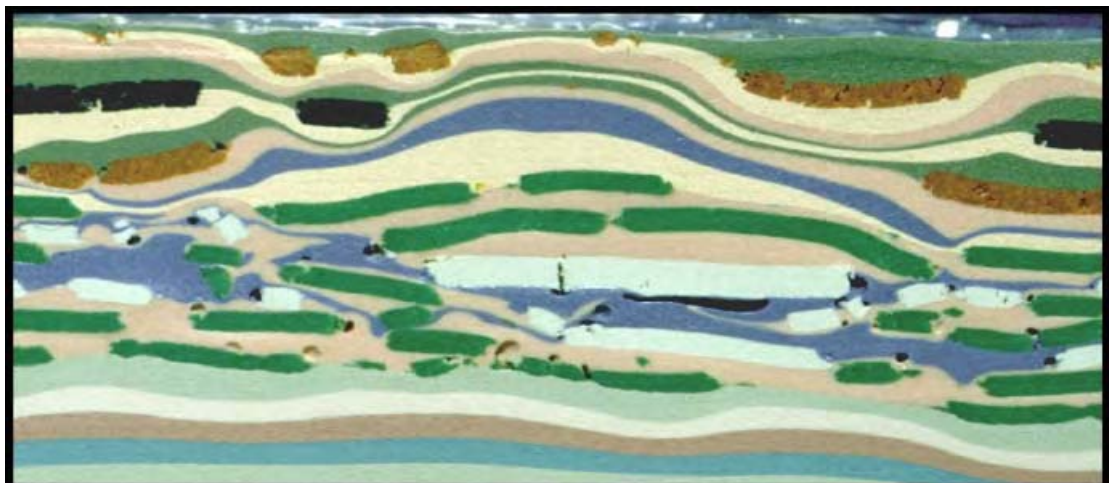
Figure 63: Illustration of centrifuge modelling of upright antiforms (domes) developed during extension. These may be viewed as analogues for the development of the granite-cored such as Mt Margaret, Raeside, and Lawlers. The development of the folding is not diapirism, but gravitational instability facilitated rising batholiths in an extensional environment.
