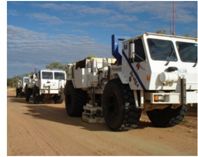
Figure 2. IVECO Hemi60 Vibroseis trucks working along traverse 01GA-IG1. The trucks generated seismic waves by sending small vibrations into the ground. The vibrations are reflected off changes in rock.
