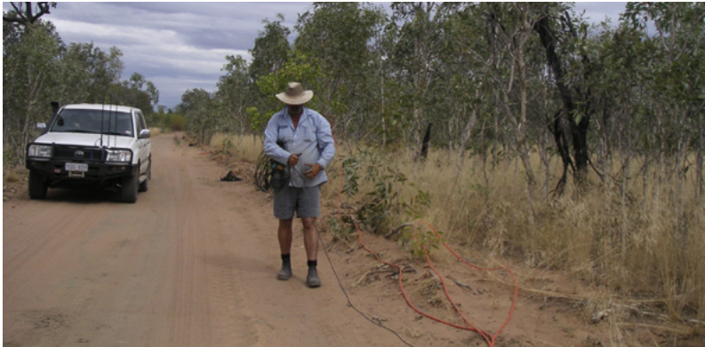
Figure 3. Terrex seismic crew laying out the geophones to record the reflected seismic waves along traverse 01GA-IG1.
