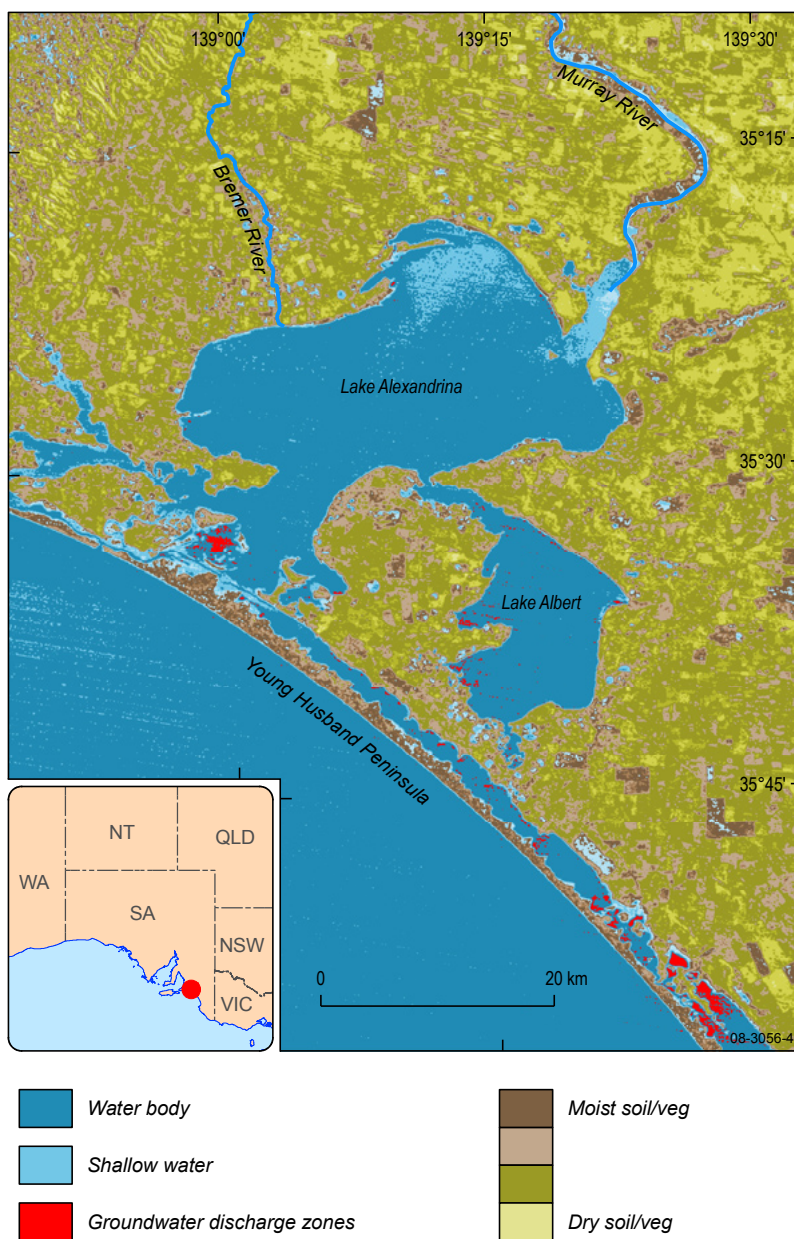
Figure 4. Thermal based classification of the Coorong and Lower Lakes region. Red areas are groundwater discharge zones.
