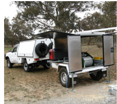
Figure 1. The new geothermal borehole logging equipment during a field test.
