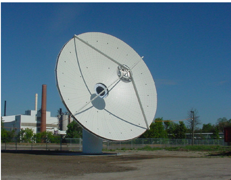
Figure 2. AuScope Patriot 12 metre VLBI telescope dish to be installed at Katherine, Northern Territory and Mingenew, Western Australia.
