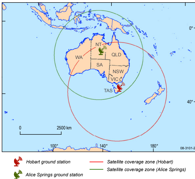
Figure 1. Surveillance areas monitored from Geoscience Australia's ground stations at Hobart and Alice Springs.
