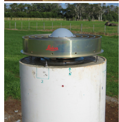
Figure 1. Typical AuScope GNSS installation at Norfolk Island collocated with Australian Tsunami Warning Service (ATWS) seismograph station.
