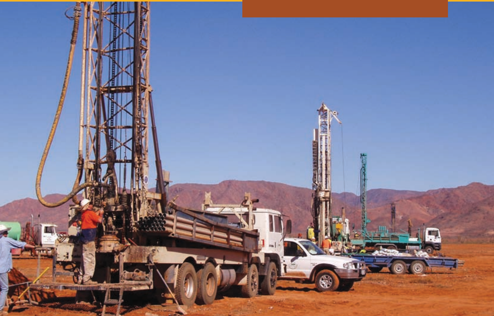
Exploration drilling (rotary mud drill rigs) at Four Mile uranium deposit, Frome Embayment, South Australia (Alliance Resources Ltd)
