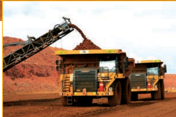
Surface miner loading haul trucks at Cloud Break iron ore mine, Western Australia (Fortescue Metals Group Ltd).
