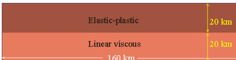
Figure 8-10: Initial geometry of a two-layer crust deformation model.
