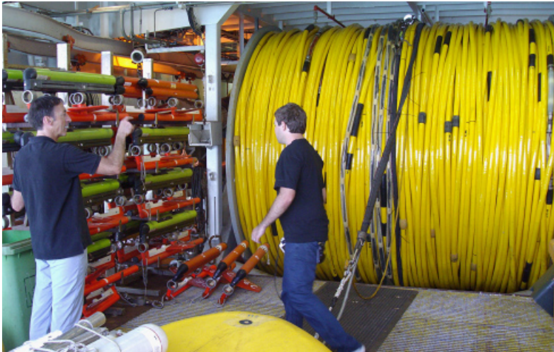
Figure 1. The 8 kilometre solid streamer, tail buoy and stabilizer ‘birds’ being inspected prior to the start of the Southwest Margin 2D seismic survey.
