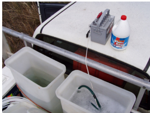
Figure 24: Soaking pump and sample tubing in bleach (container on right), with rinse container on left (photo courtesy of UNSW Water Research Laboratory)
