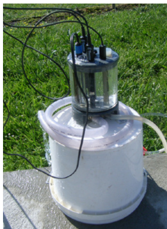
Figure 12: Flow cell used to monitor field parameters during pumping
