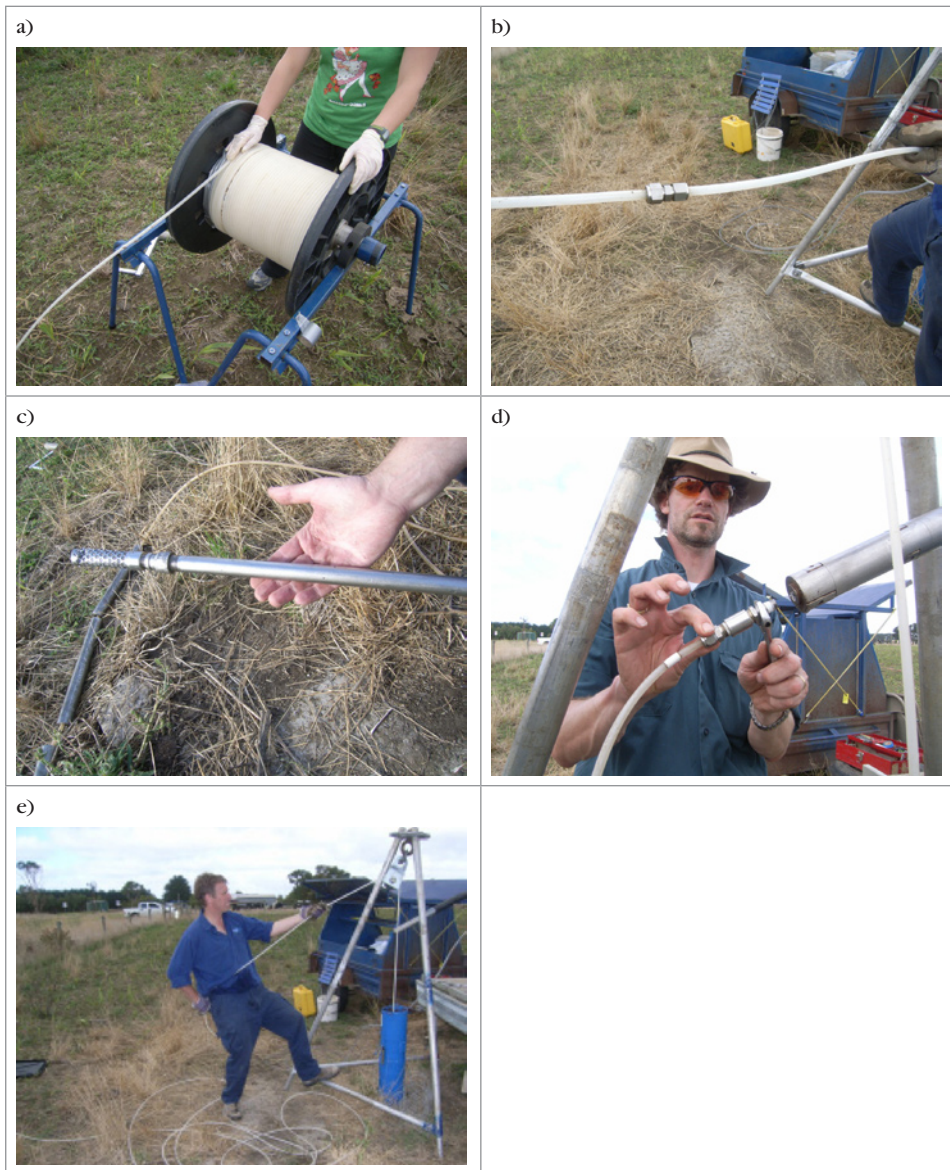
Figure 11: Deep groundwater sampling equipment: a) reel of LDPE tubing; b) connection between lengths of tubing; c) intake screen with weights in background; d) connecting the tubing to the pump; and e) tripod and swivelling block used to lower and retrieve tubing
