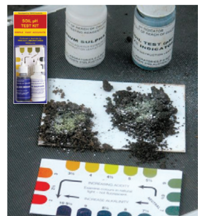
Figure 1. Field sampling at the point of collection: Inoculo™ field pH kit (inset) and measurement of the pH of two soil samples.
