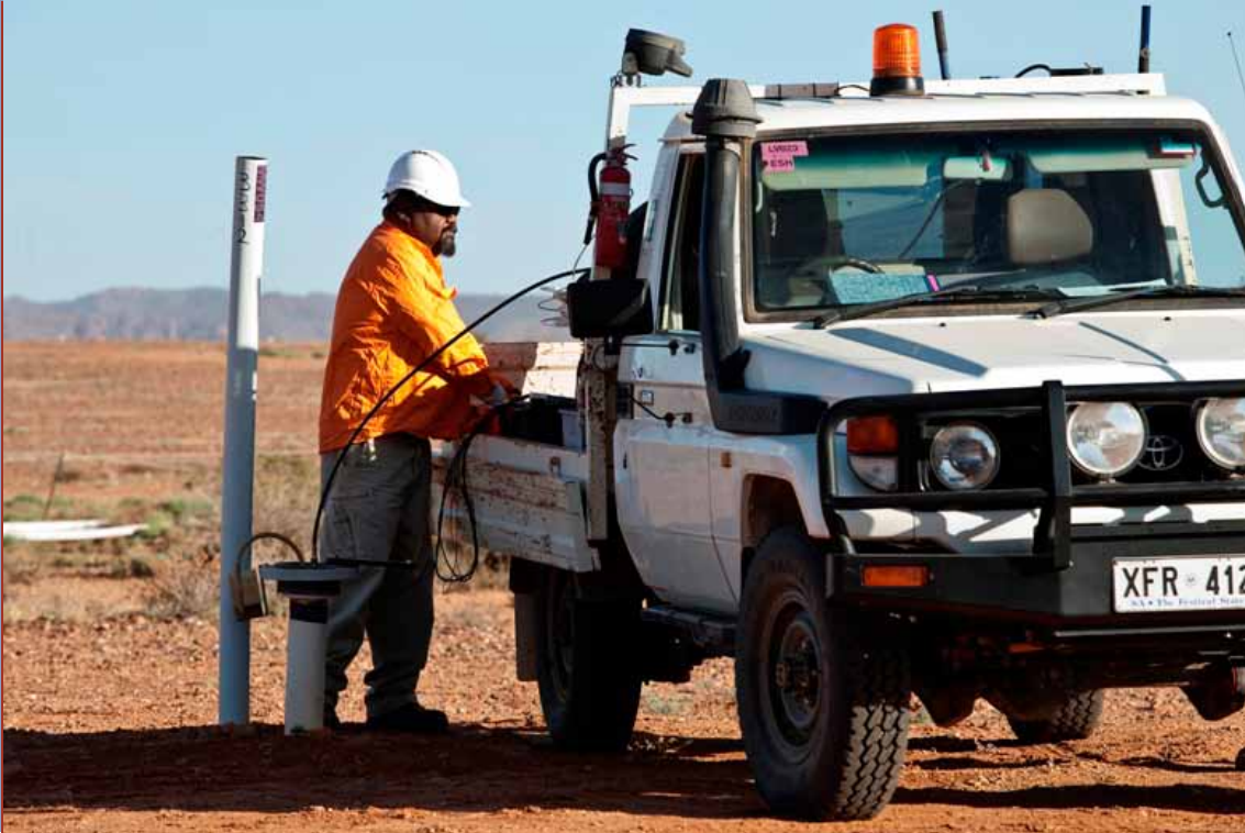
Monitoring groundwater quality at Beverley in situ recovery uranium mine, South Australia (Heathgate Resources Ltd)
