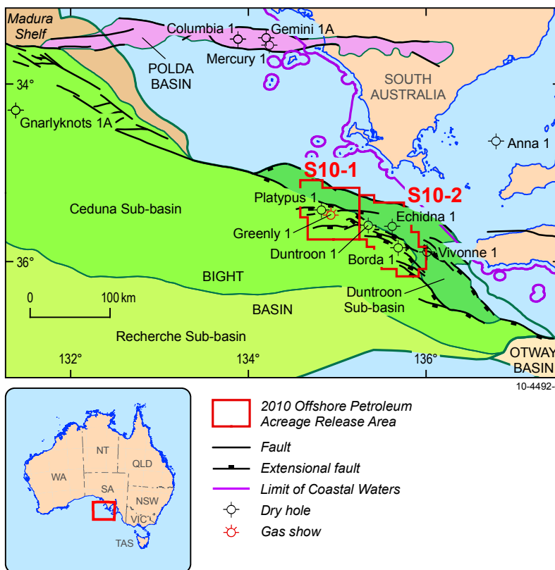
Figure 6. Structural elements of the eastern Bight Basin showing 2010 Release Areas and wells drilled.
