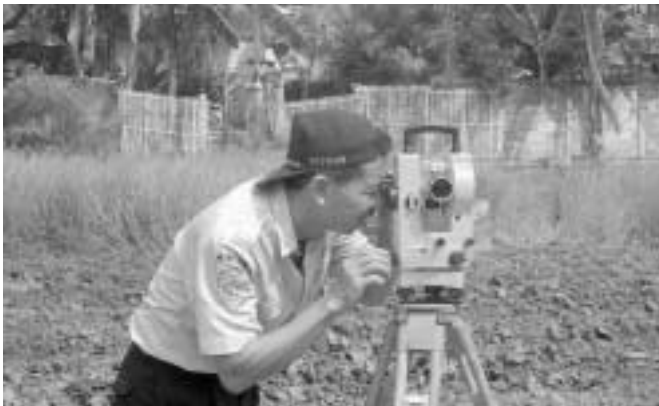
▲ Ibrahim Limer, of Indonesia's BMG, takes magnetic measurements at Tangerang observatory with one of the new absolute magnetometers provided as part of the GSLP projects.
