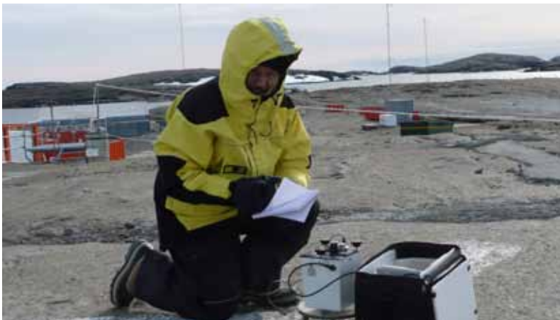
Figure 1. Ties between existing gravity base stations and the new absolute gravity base stations were conducted using a relative gravity meter.
