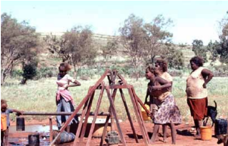
Figure 2. CAT hand-pump of the type installed at Winner's Bore. The durability of these hand-pumps stems from their occasional use compared to the near continuous operation cycles of similar flush cap pumps used for windmill-operated systems (photo courtesy of Dr Bruce Walker).
