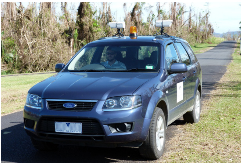
Figure 1. The Rapid Inventory Collection System vehicle gathering data in north Queensland in the aftermath of Cyclone Yasi.
