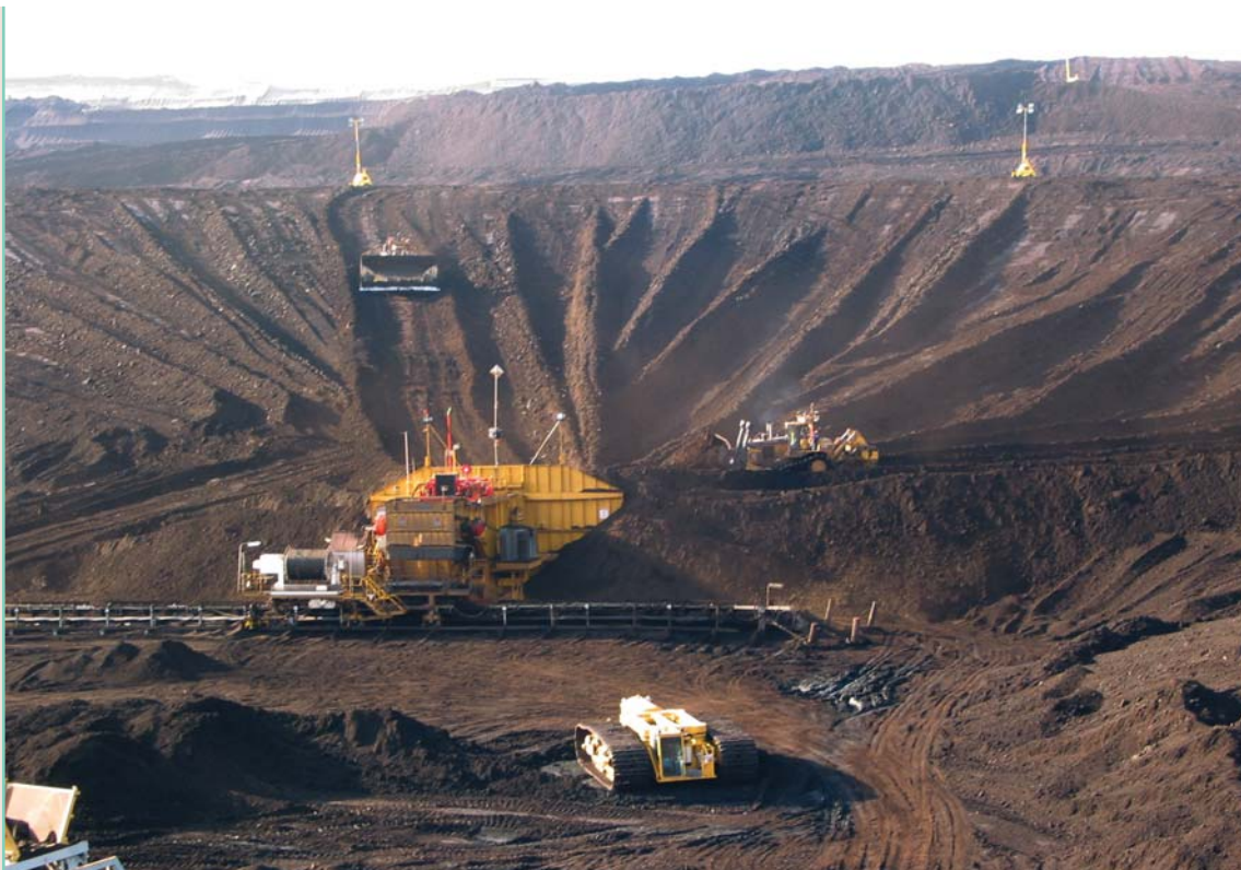
Satellite guided D11R dozers using the radial sector method to push coal to a feeder-breaker at the Yallourn brown coal mine, Victoria. (Yallourn Mine Alliance, Roche Thiess Linfox Joint Venture)
