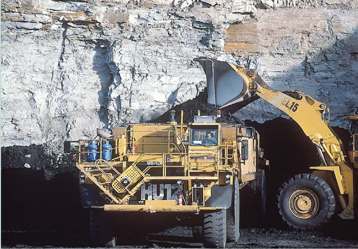
Loading a coal haul truck at the Moura mine, Bowen Basin, Queensland. (Anglo Coal Australia)
