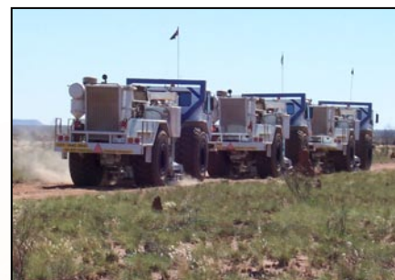
▲ Figure 2. ANSIR (through Terrex Seismic Pty Ltd) seismic acquisition in operation in the Tanami with three IV1 60 000 lb vibrators operating on traverse 05GA-T2 to send signals through whole of crust and back.
