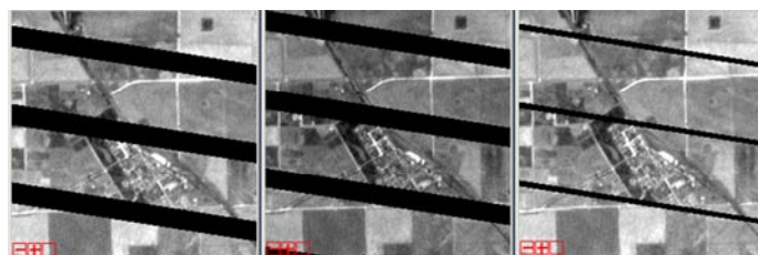
▲ Figure 2. Combining two SLC-Off scenes. The edge portion of a primary SLC-Off scene acquired on 2 March 2004 (left), an SLC-Off fill scene acquired on 18 March 2004 (middle), and the composite product generated from these two scenes.
