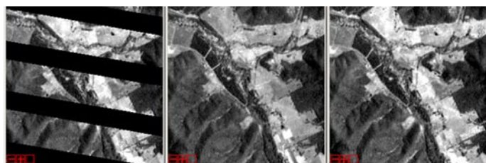
▲ Figure 1. Combining SLC-Off and SLC-On scenes. The edge portion of a primary SLC-Off scene (left), an SLC-On scene with equivalent seasonality (middle), and the composite product generated from these two scenes.
