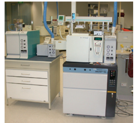
▲ Gas chromatography – stable isotope mass spectrometer used in hydrocarbon isotope analysis.
