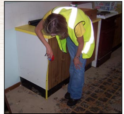
▲ Figure 1. Surveying water depth in residential dwellings.
